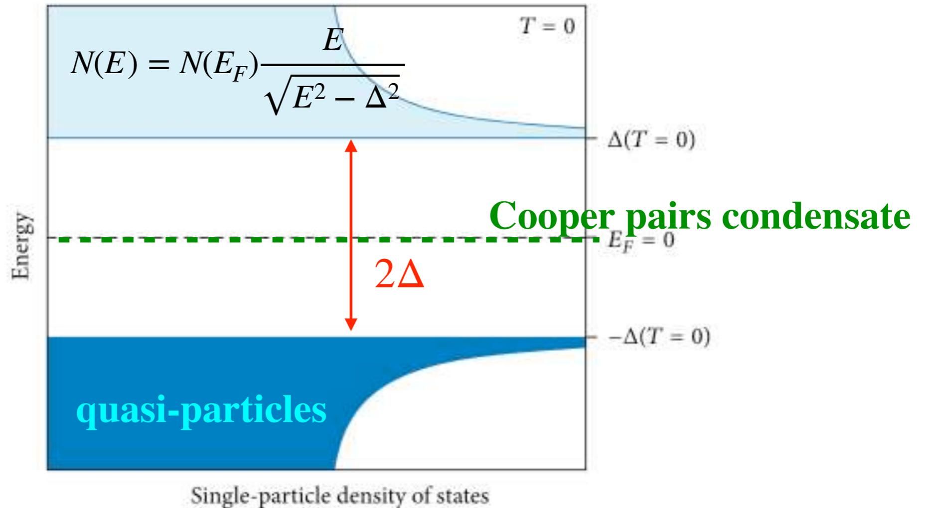
The gap protects the SC-condensate from thermal/photon excitations
