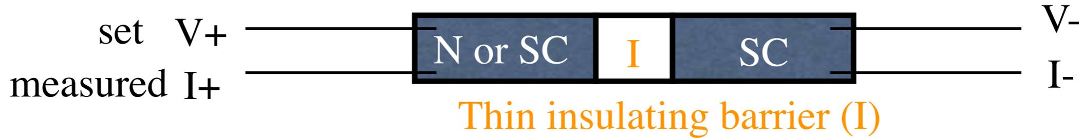
Tunneling, i.e current when the voltage set is larger than:
