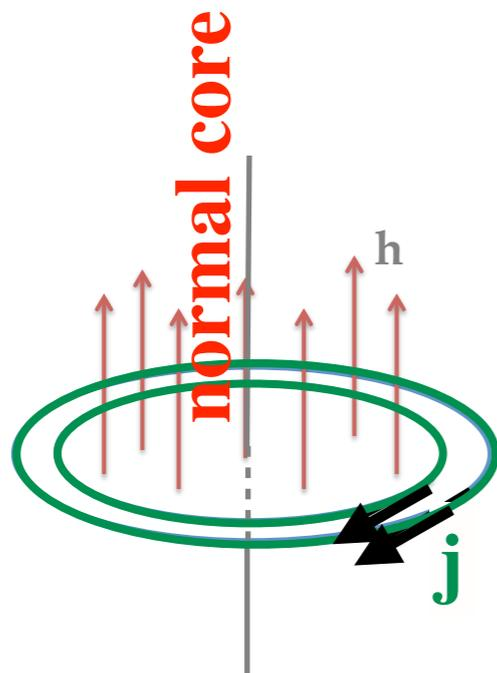
**Supercurrent** circulates around the **normal** (i.e. non-superconducting) core of the vortex.
