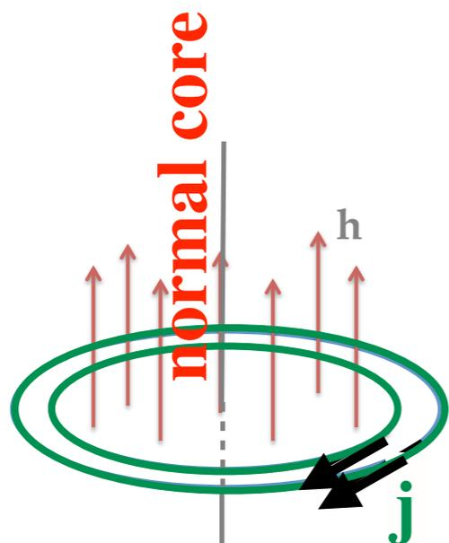
**Supercurrent** circulates around the **normal** (i.e. non-superconducting) core of the vortex.
